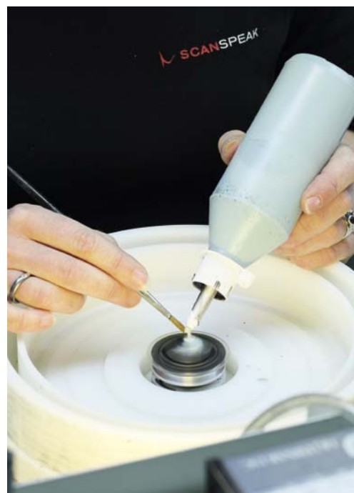
Hand coating of dome tweeter textile diaphragms. Each diaphragm is individually coated for optimum performance.
