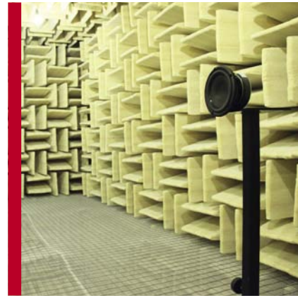
Scan-Speak engineering facilities include: 2 large anechoic chambers, each 6 x 7 x 8 meters.
