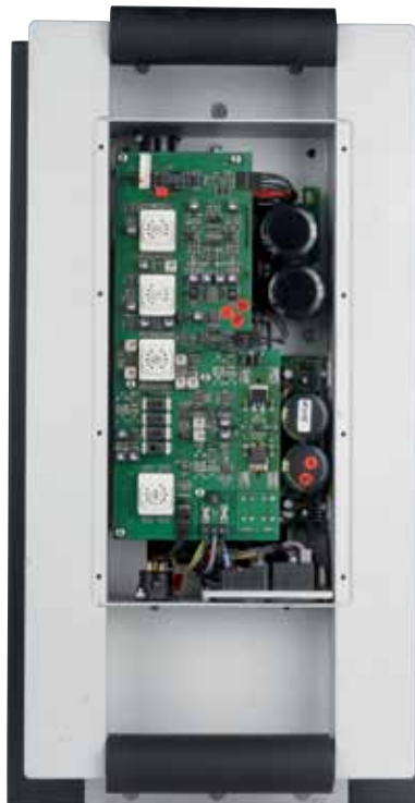
Active to the max: High-capacity Class-A/B power amplifiers drive the speakers and deliver excellent sound quality.
