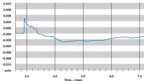
**Step response:** Just about perfect and without any trace of post-oscillation. The instantaneous rise and the optimum addition of the MSW and woofer means that the finer details are never missed.
